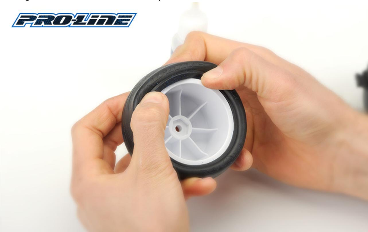
Your tire and wheel are ready to come together. Push the tire over the wheel and seat the beads. Remember to check the orientation for directional tires. When the tire bead appears to be properly aligned between the rim's mounting flanges, give the assembly a spin to make sure it is true and realign as needed.
