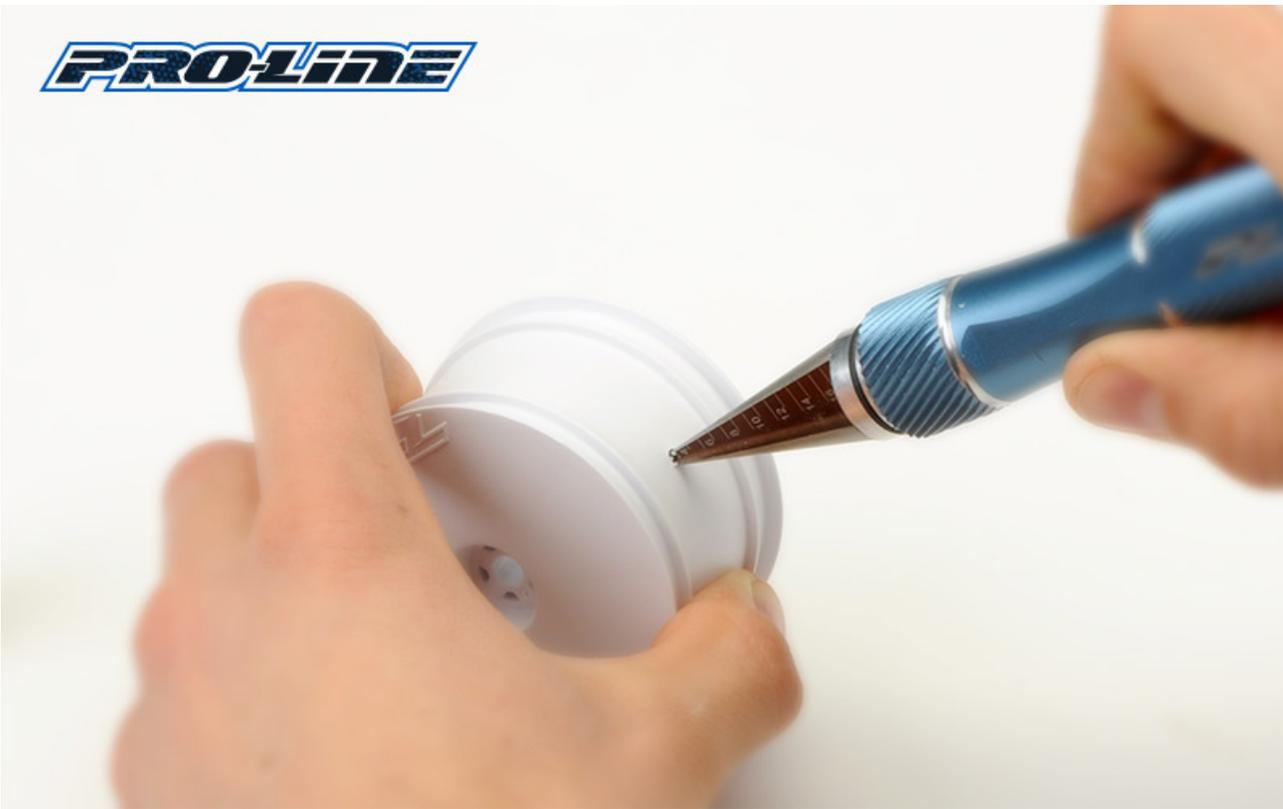
Proper tire ventilation will yield the best and most consistent traction. Using your reamer or hobby knife, carefully ream two holes on opposite sides of the wheel. These are pre-marked on Pro-Line wheels. This will allow the tire to "breathe" when running on rough surfaces or landing off of big jumps.
