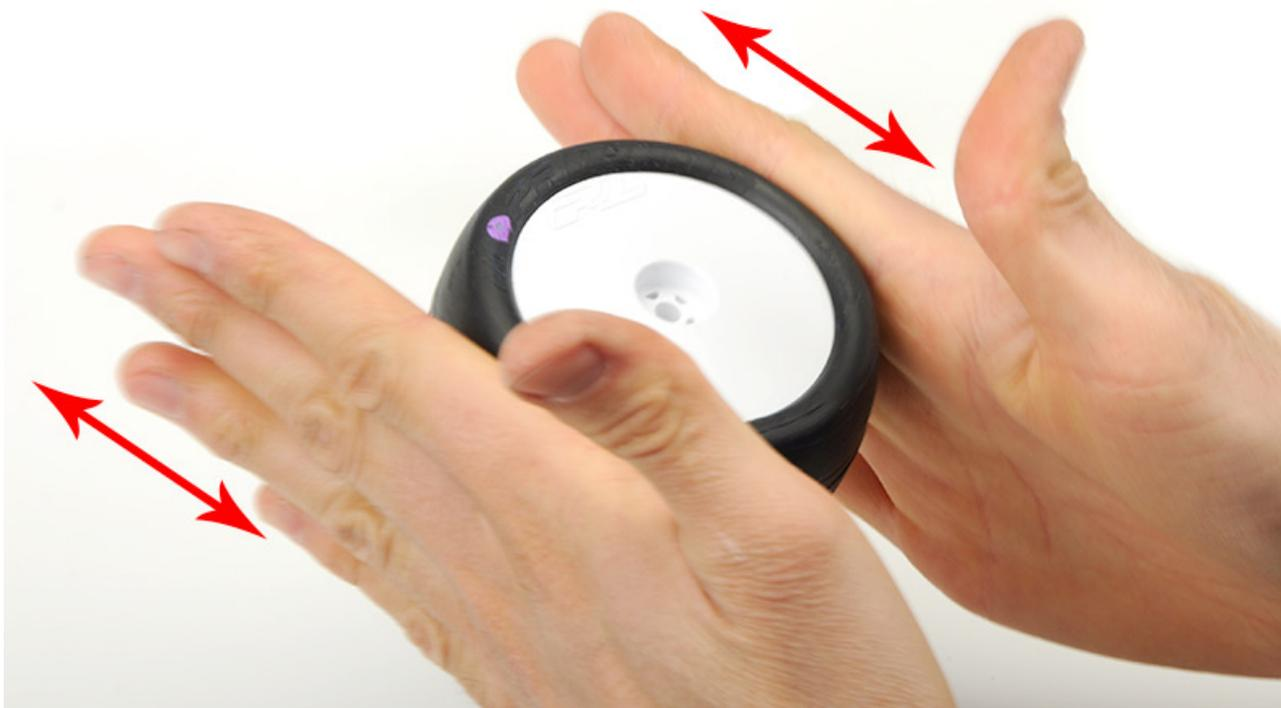
With the foam inserted and the tires in place on the wheel, roll the tire back and forth between your hands in to check the foam and tire bead are properly seated onto the wheel.
