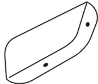
.....-These spill plates can be located directly over the wing stands or wherever they are found to be most effective. The inner spill plates are to make the rear wing slightly more efficient.
