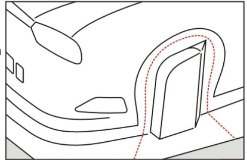
.....-After careful trimming, these pieces can be mounted into the rear wing with the supplied screws/nut, servo tape, or Shoe-Goo. As with most other wings, you have the option of trimming the entire piece down following the inner trim lines.
