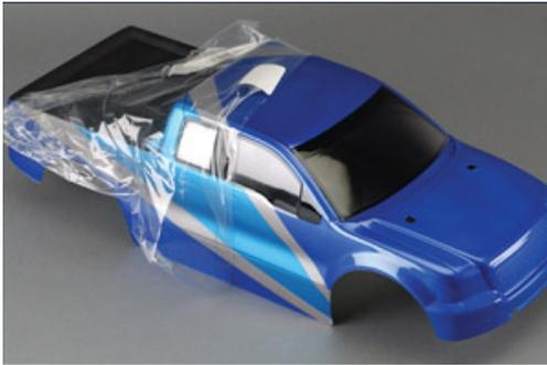
Peel back the protective film, and remove the window masks.
