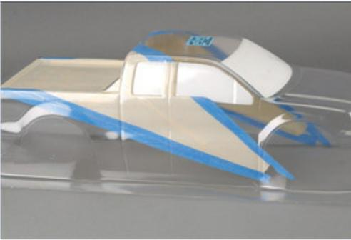
Fill in the area you want to paint with your second color. I used blue and beige tape to show the separate paint sections. Painting from dark to light is ideal, so leave the darkest section clear, and paint this first.
