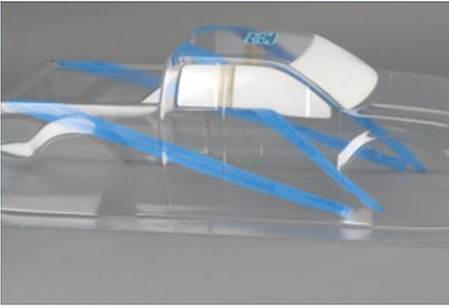
This paint scheme is quite simple, and uses straight masking tape for the design. Make sure you use high quality masking tape, and press down all the edges. First mask off the color that you want to paint last.
