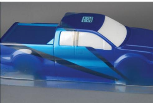
Again spray light coats and cover evenly. You can then back it with white or silver, but in my case I will use silver for the stripes, so no need to back it separately. When the paint has completely dried remove the taped stripes.
