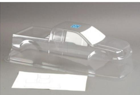
Using the molded in window lines as a guide apply the window masks to the inside the body. Be sure to press down all the edges to keep paint from sneaking under. The masks keep the windows clear while you paint.
