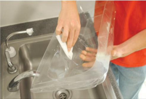
To remove any residue left on the body after molding, you must wash it inside and out. Use warm soapy water in your sink, paying special attention to the tight curved areas and corners. Dry the body with a clean towel or hair dryer. It must be completely dry before you paint it.
