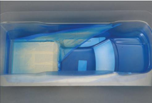
For your first color, spray a light even coat and allow to tack up. Then apply a second light to medium coat to fill in your color. If another coat is required, apply lightly as to not create build up on the design masking tape. This would result in a difficult removal of the tape edge.
