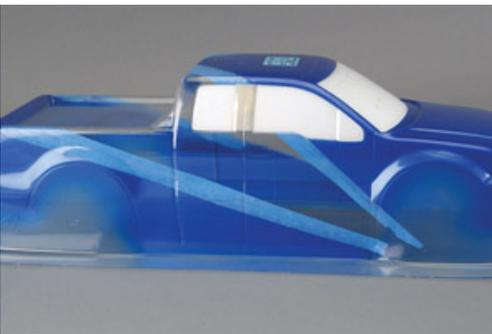
When your first color has completely dried, unmask the second section of the paint scheme. While removing the tape, watch that you don't remove any of the stripes accidentally.
