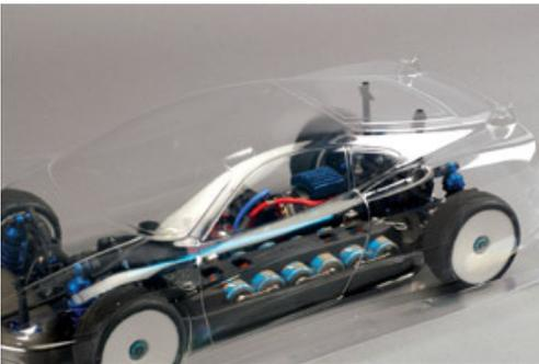
If your body does not have mounting holes marked for your chassis you can mark them before you paint. Drop the body over your chassis, center it and use a permanent marker to mark the body posts. You can also mark the wheel wells. Touring car and On-Road bodies sometimes have no rear wheel well outlines, this give you freedom to make a perfect fit for your chassis. (Touring Car body shown)
