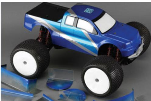
Trim out your body using curved scissors for the wheel wells and straight scissors for the lower lines. Drill out your body post markings with either a Dremel tool or reamer. The protective film will help keep your body from getting scratched as you cut and drill.
