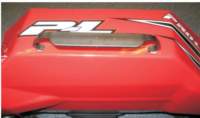
7. Re-attach the front bumper and your ready to go. The sides of the undertray can be cut to any size depending on preference.
