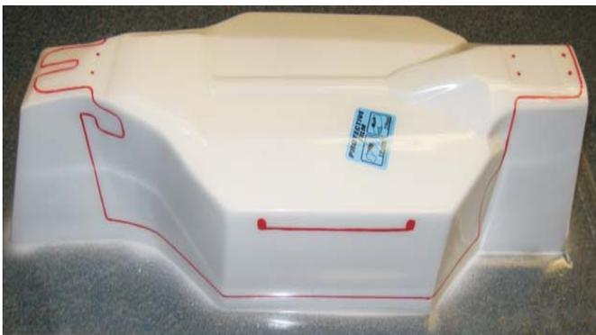
1. Using Lexan scissors cut along the scribed lines and Remove the excess material from the undertray. ( illustration #1)
